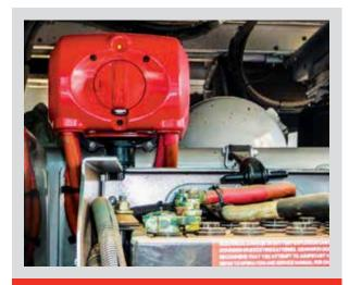
The BMIS has a current rating of 400A continuous current with a 3500A cranking capacity, which makes it unique.
