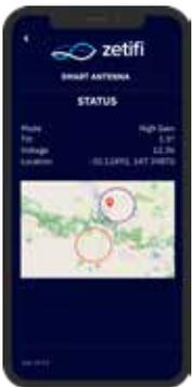
The companion app connects to your smart antenna via bluetooth and enables real-time updates of pre-loaded terrain maps or manual selection of high or low gain modes.
