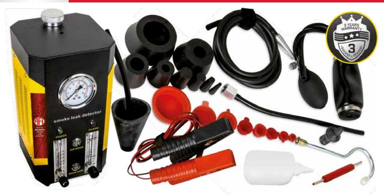
The TO90206 AFi Diagnostic Smoke Machine features a flow meter and pressure gauge. The air pressure is adjustable between 0-15psi to suit multiple test situations, for example higher pressure for turbo systems, lower pressure for crankcase breather testing.
