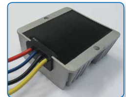
Fully sealed and potted (IP68)
