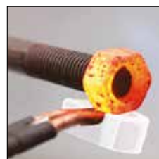
Releasing of rusted bolts
