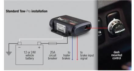
The remote head control is mounted in the dash of your vehicle and the electronic module is mounted out of sight, making the Tow-Pro ideal for vehicles fitted with knee or lower leg airbags.
