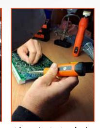
A fast re-charging time of under 60 seconds, provides up to 45 minutes working time and a maximum temperature of 450 degrees Celsius gets the job done.
