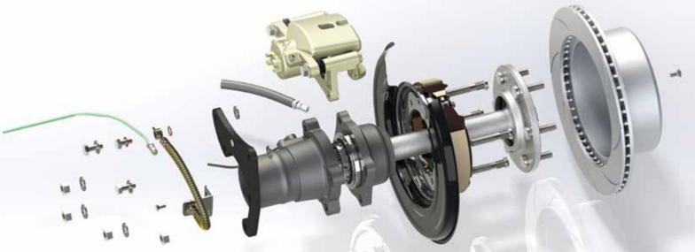
\*Independent Australian engineering (including electronic stability control) test results proved that at 100kmh the HULK 4x4 rear disc braking system upgrade stopped on average 32m sooner than the original equipment. A fantastic result that enhances load carrying and towing performance. Official test at vehicle GVM+ weight of 3590kgs.
